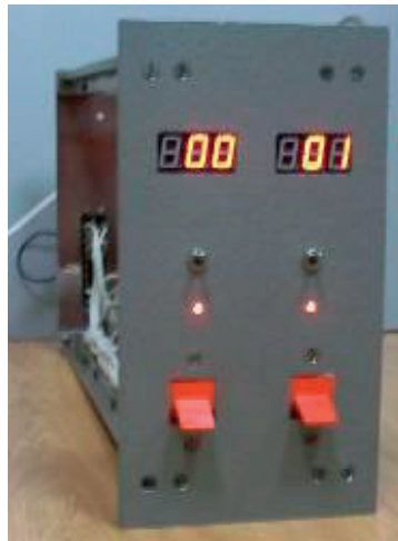
FIG. 18. Unit for remote control of turbomolecular pump of the injector and the analyzer.
