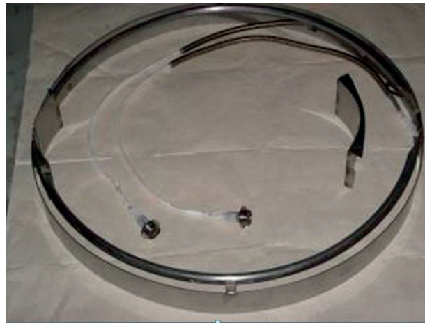
FIG.30. External view of the system with a set of 16 Mirnov coils.
