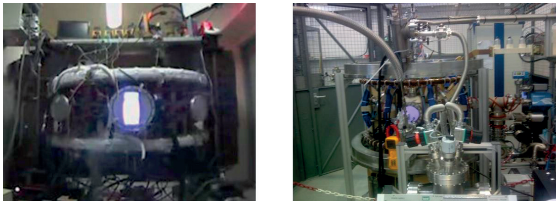
FIG. 1. First application of HTS in tokamak magnets: GOLEM August 2011, left; ST25 2.5 sec plasma discharge, 4 October 2013, right. Reproduced from Ref. [1] with permission.
