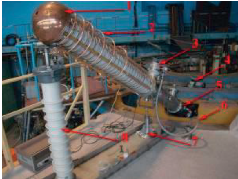
FIG. 13. Injector part of the diagnostic complex. 1 - shield of emitter block, 2 - security rings of the accelerator tube, 3 - turbomolecular pump TV-301, 4 - vacuum valve, 5 - primary beam-line of the blocks of deflecting plates ( \alpha_1 - \beta_1 , \alpha_2 - \beta_2 ), 6 - backing tract, 7, 8 – support and HV insulator.
