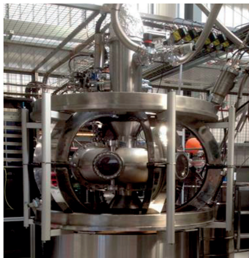
FIG. 6. ST25(HTS): world's first all-HTS tokamak.
