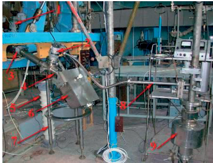
FIG. 14. Analyzer part of the diagnostic complex. 1 - valve («Uragan-2M»/analyzer), 2 - turbomolecular pump TV-301, 3 - the first block of the air-bellow for the alignment of the analyzer, 4 - second air-bellow block, 5 – isolator of secondary beam-line, 6 - energy analyzer, 7 - support of the analyser, 8 - backing tract, 9 – vacuum trap with liquid nitrogen.
