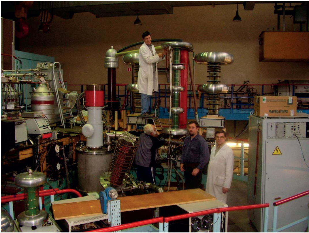
FIG. 1. HIBP on the diagnostic platform of the T-10 tokamak. Installation phase.
