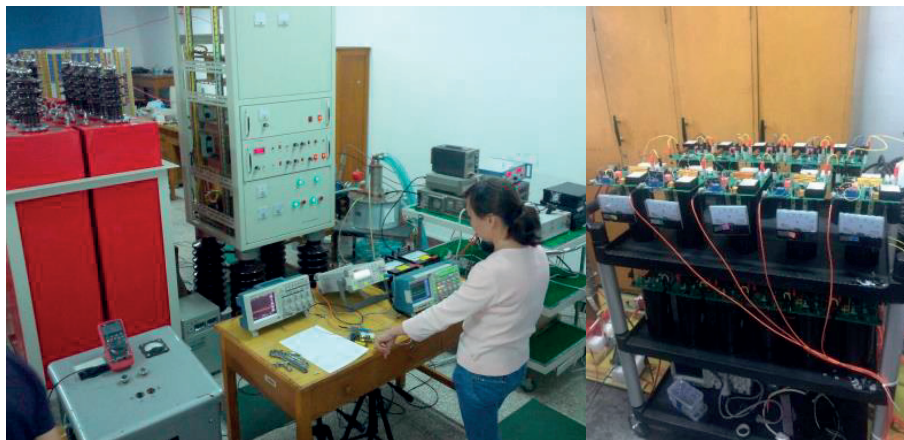
FIG. 8. The klystron (left) and 20 modules of the PSM power supply (right) under test.
