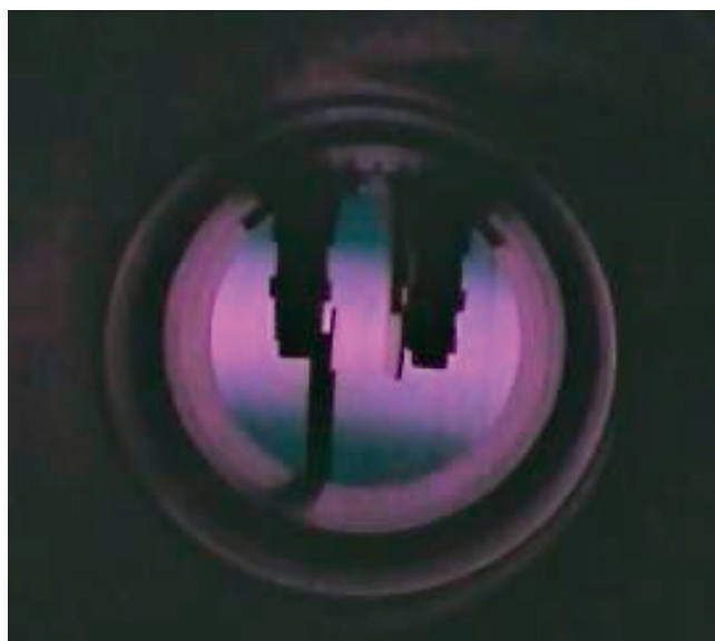
FIG. 3. Photo of RF discharge in helium made through side window.
