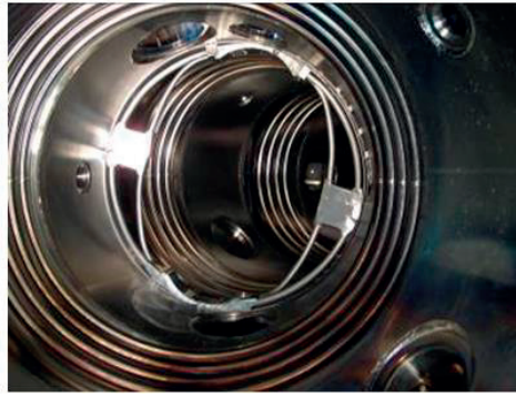
FIG. 26. Side view of diamagnetic loops installed in U-2M vacuum vessel.
